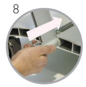
Slide each curved profile into opposite ends of the central channel ensuring uprights arc away from column.
