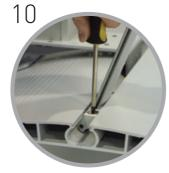
Ensure uprights are positioned centrally and tighten pre-located screws (two per upright). Replace both side trim mouldings.
