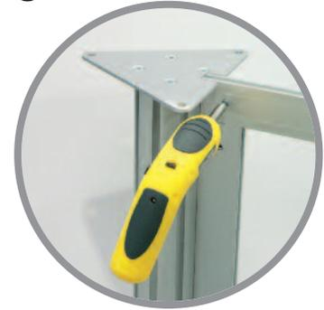
Attach second curved profile to both posts and both verticals ensuring the top of the profile is flush with the top of the triangular stealth plates. Tighten clamp screws to secure in place.
