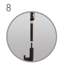
Raise pole with attached graphic and align bottom of pole with protruding pin of base. 9
