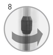
Unlock the telescopic pole by twisting the handle anti-clockwise
