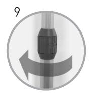
Extend the telescopic pole to tension the graphic and twist handle clockwise to lock into position
