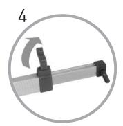
Flip up catch on the graphic rail (affixed to base unit) and extend to the required length to suit graphic width
