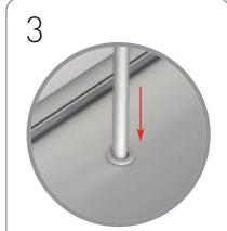
Insert bottom of the pole into the pole plug in base, ensuring it is fully located.
